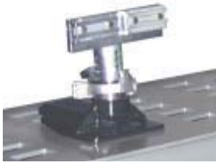
Height adjustable clamping system securely anchors vehicle to rack platform
