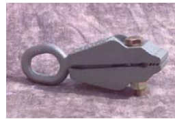
0300 Jr Clamp Gripping Surface: 1½" wide (38 mm), ¾" deep (19 mm) Overall Length: 9" (229 mm) Weight: 5 lbs (2.27 kg) Capacity: 5 tons (4,536 kg)
